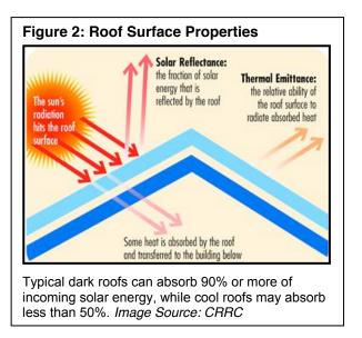
increase the heat flow into the building, causing the air conditioning system to work harder and use more energy in summertime. In contrast, light-colored roofs absorb less than 50% of the solar energy, reducing the roof temperature and decreasing air conditioning energy use.
